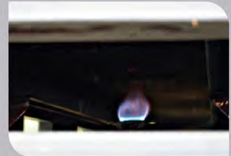
Figure 9 Flame characteristic of gas burner when observe at side observation window
