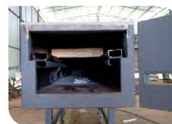
Figure 7 Internal characteristic and gas burner of test apparatus
