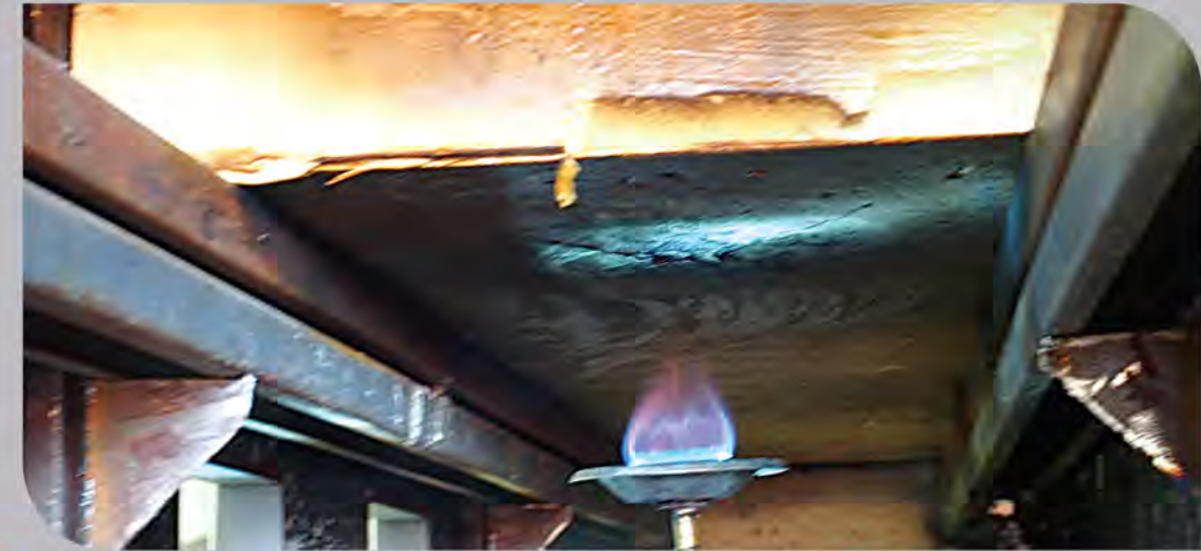
Figure 8 Burning characteristic of flame spread when observed at front observation window
